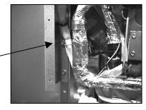
7. Install wire ties, spacing them as shown in the illustration on reverse. Use additional ties as required to secure wiring bundles so that they remain clear of the frypot and oil return line, with no tension on the connectors. When finished, no wire bundles should pass inside or contact the shields or springs.
